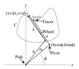
**Figure 3.** The motion of the tracer arm of a polar planimeter as it traverses a curve C counterclockwise. The tracer arm is attached via a pivot to an arm with a fixed pole at the origin. This pivot traces out a circular arc of radius b as the planimeter traces out the curve.
