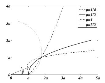
**Figure 7.** Graphs of tracks for planimeters that will integrate  $(g \circ f)(\theta) = f(\theta)^p$ , corresponding to  $\beta(r) = \sin^{-1} \frac{(r-a)^p}{r}$ .
