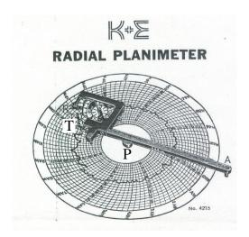
**Figure 4.** Diagram from the instructions to a Keuffel and Esser radial planimeter (shown with a circular chart) in the author's collection. P marks the pivot and T marks the tracer. The tracer arm AT can slide as well as turn on the pivot.
