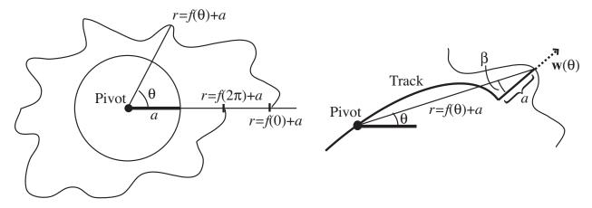
**Figure 6.** Diagram for designing a more general planimeter like those shown in Figure 5. In general, r is the distance from the pivot to a point on the curve.
