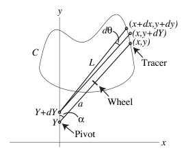
**Figure 2.** The motion of the tracer arm of a rolling planimeter as it traverses a curve C counterclockwise. The tracer arm is attached to a roller which rolls along the y-axis. The tracer arm may pivot where it attaches to the roller at (0, Y) as the tracer at its opposite end traces out the curve with coordinates (x, y).
