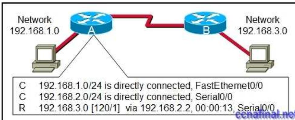
Refer to the exhibit. The output is shown for the show ip route command executed on Router A. What does the IP address 192.168.2.2 represent?
