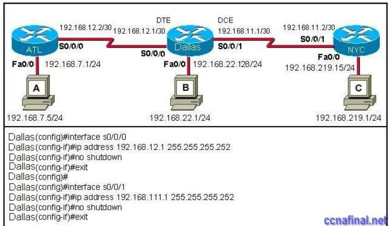
Refer to the exhibit. A student is responsible for the IP addressing, configuration and connectivity testing of the network shown in the graphic. A ping from host B to host C results in a destination unreachable but a ping from host B to host A was successful. What two reasons could account for this failure based on the graphic and partial router output for the Dallas router? (Choose two.)
