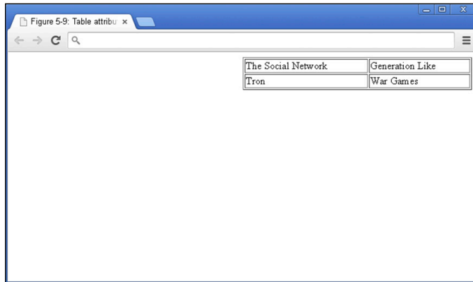
Figure 5-9: A table with deprecated align , width , and border attributes.
