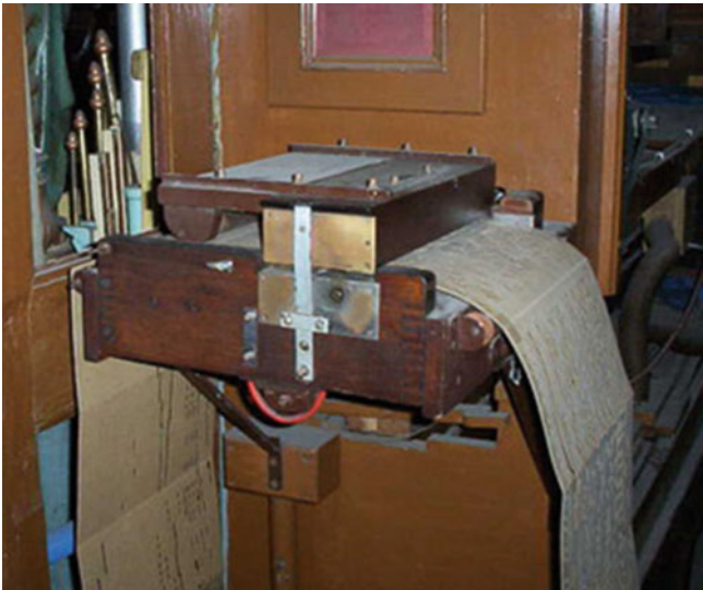
Fig. 1.2 The Gavioli 87 Keyless Military Band Organ uses bursts of air to read the holes, instead of metal keys
