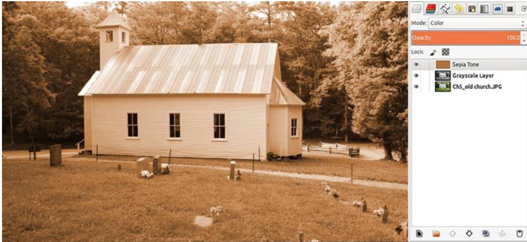
**Figure 5-11.** Sepia tone applied to a layer set to the color blend mode
