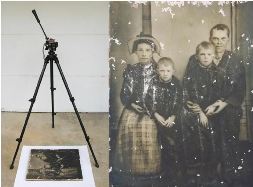
**Figure 2-3.** A tripod set up as a copy stand and a 16" × 20" portrait digitized with a camera
