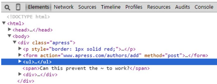
Figure 3-11. Selecting all the p elements that are siblings of the ul element
