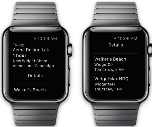
Figure 3.61. Example UI for full Watch application that displays additional details for the user. The user can scroll down to see additional information
