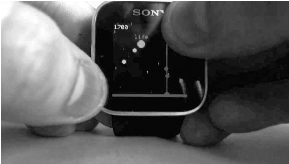
FIGURE 1-1: Sony SmartWatch v1 hacked to be programmed using the Arduino IDE by Arduino Verktad (image by Asier Arranz)
