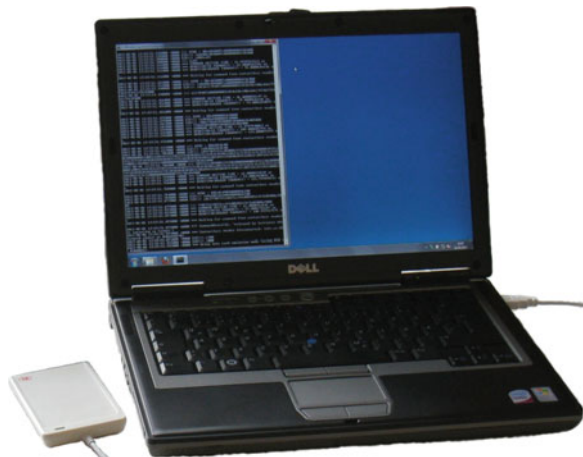
Fig. 6.9 Card emulator made from a notebook and an ACS ACR 122U NFC reader (Source [25])
