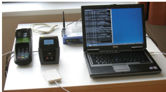
Fig. 7.1 Test setup for performing a payment transaction with the card emulator at a POS terminal (Source [15, 17])
