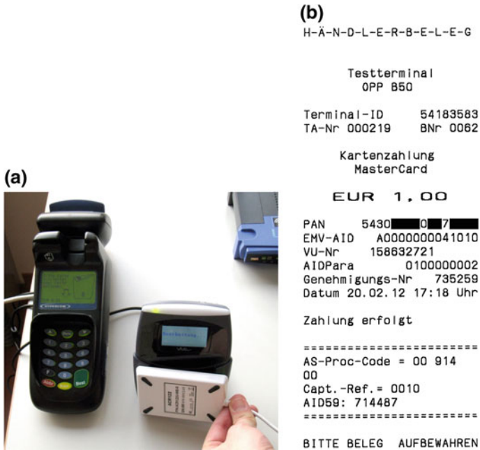
Fig. 7.2 Performing a successful payment transaction with the card emulator at a POS terminal: a payment transaction in progress (Source [15]), b payment receipt
