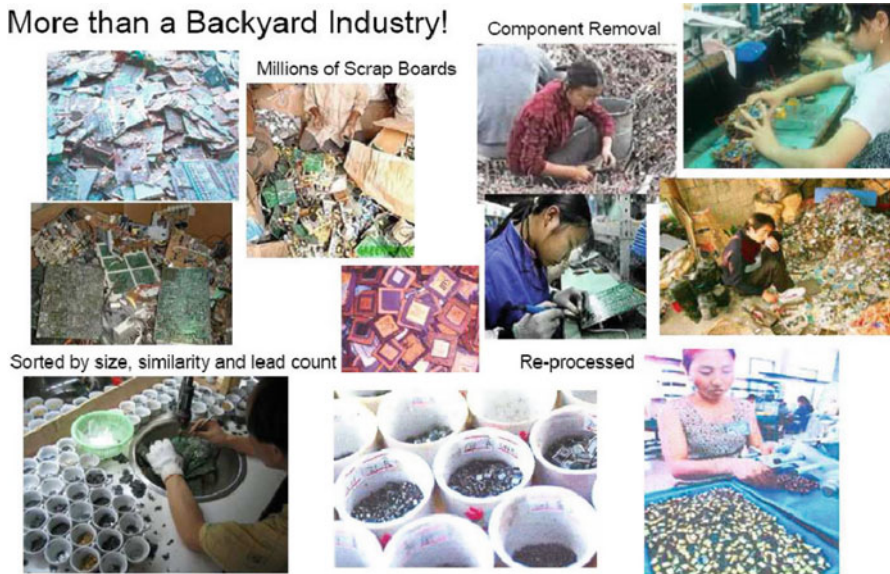
Fig. 2.3 A typical IC recycling process [27]
