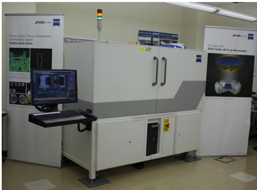
Fig. 4.4 Zeiss Xradia 510 Versa: X-ray imaging system (CHASE Center, University of Connecticut)
