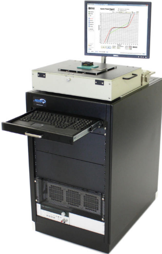
Fig. 5.3 A typical curve tracer by National Instruments
