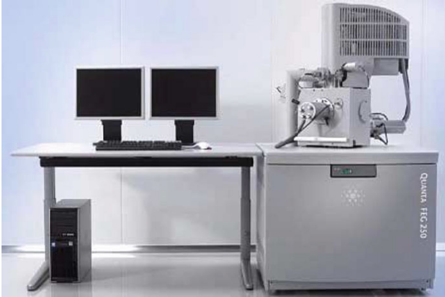
Fig. 4.7 FEI Quanta 250 FEG field emission scanning electron microscope (center for Clean Energy Engineering, University of Connecticut)
