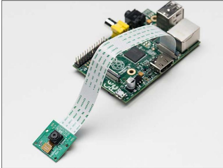
Camera module connected to Raspberry Pi
