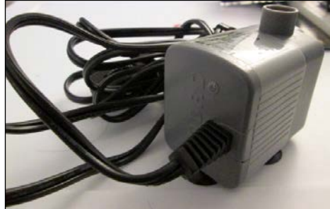
Fountain pump to be placed inside the basin
