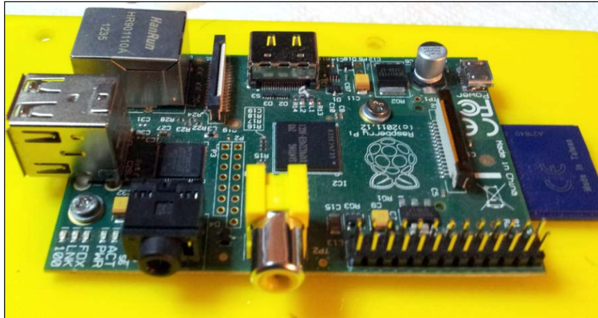
Raspberry Pi mounted using M2.5 screws
