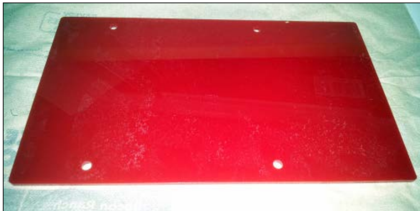
A top plate used to mount the battery of the line following robot
