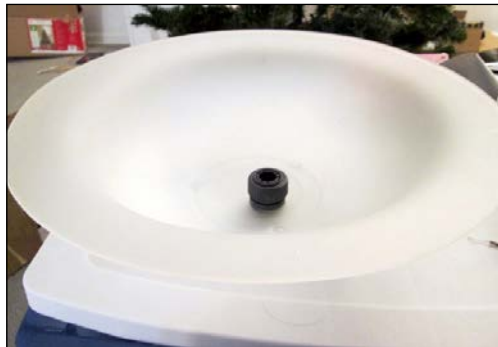
A basin with a sealed electrical outlet
