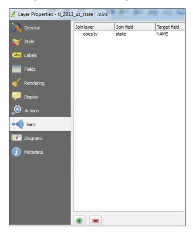
If you click on **Fields**, you will observe that some values are classified as **Strings** and some as **Real**. When we finish joining our data and saving a new shapefile, we would like the values to be identified as **Real** as this makes it easier to plot it in Tile Mill or create a cartogram.
