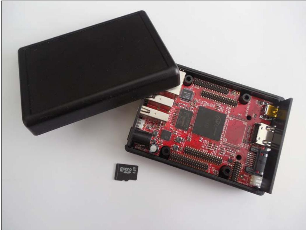
Olimex offers the A10-OLinuXino-LIME, an A10-based micro board that is marketed to compete with the famous Raspberry Pi price-wise. Due to its small size, it uses less standard 1.27 mm pitch headers for the pins, but it has nearly all of these pins exposed for use.
