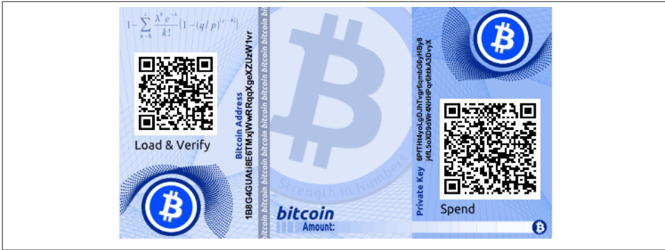
Figure 4-15. An example of an encrypted paper wallet from bitaddress.org. The passphrase is “test.”
