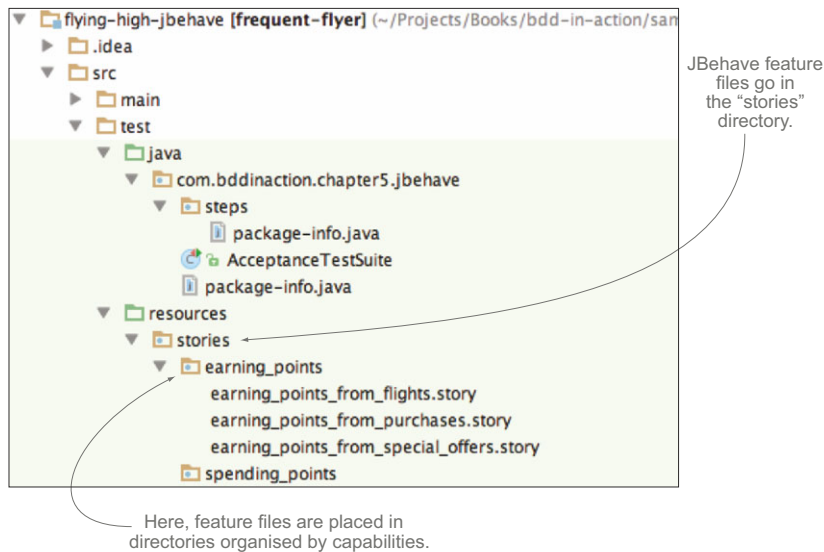
Figure 5.7 Organizing feature files into folders makes them easier to manage and navigate. In this JBehave project, the features are organized by high-level capability.
