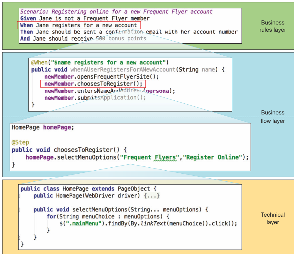
Figure 7.9 Each automation layer uses services from the layer beneath to implement a scenario.
