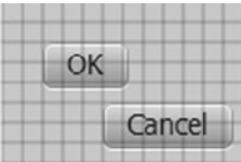
Figure 6-19. Two buttons using layoutX and layoutY properties and placed inside a Group or a Pane
