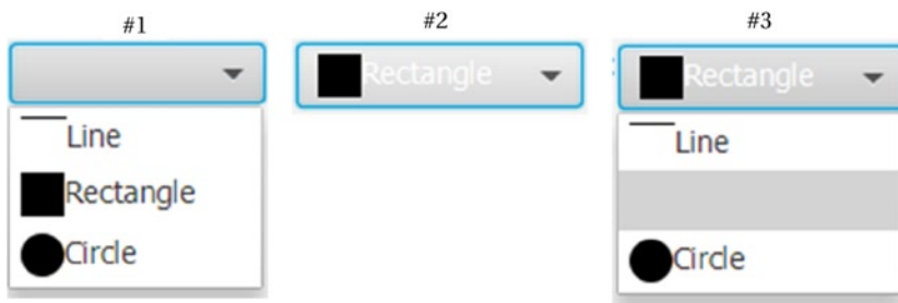
Figure 12-21. Three views of a combo box with nodes in the items list
