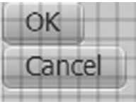
Figure 6-18. Two buttons using layoutX and layoutY properties and placed inside a VBox
