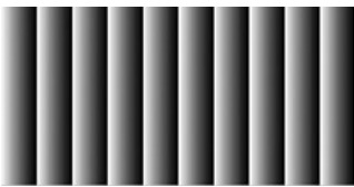
Figure 7-12. A horizontal linear color gradient with two stop points: white at starting and black at one-tenth point and REPEAT as the cycle method
