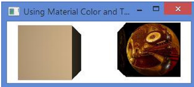
Figure 19-6. Two boxes: one with a tan diffuse color and one with texture using a diffuse map
