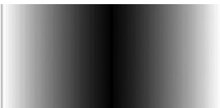
Figure 7-9. A horizontal linear color gradient with two stop points: white at starting and black at midpoint and REFLECT as the cycle method
