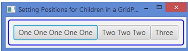
Figure 10-43. Three buttons added to a GridPane directly and then their position set
