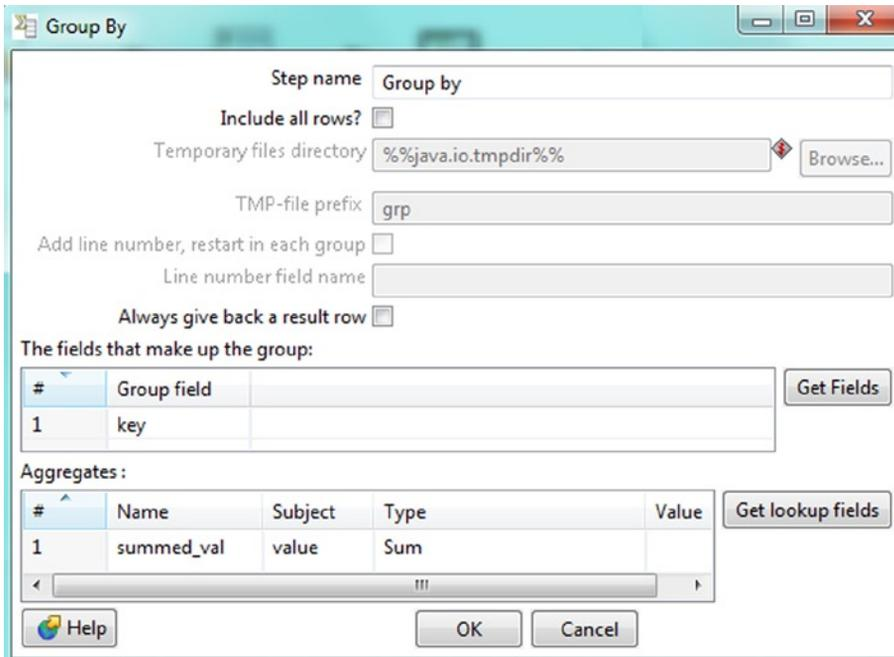
**Figure 10-13.** Group By step of reducer transformation
