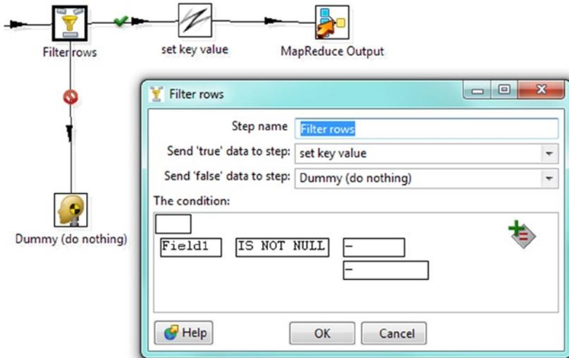
**Figure 10-8.** Filter Rows step of mapper transformation
