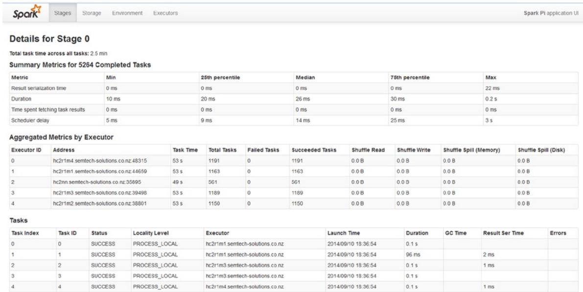
**Figure 9-8.** Spark Application interface shows job executors
