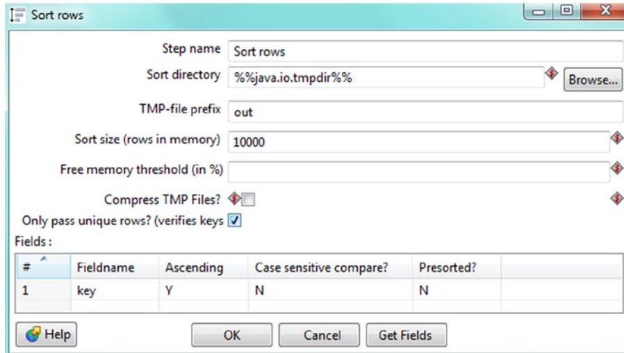
**Figure 10-12.** Sort Rows step of reducer transformation
