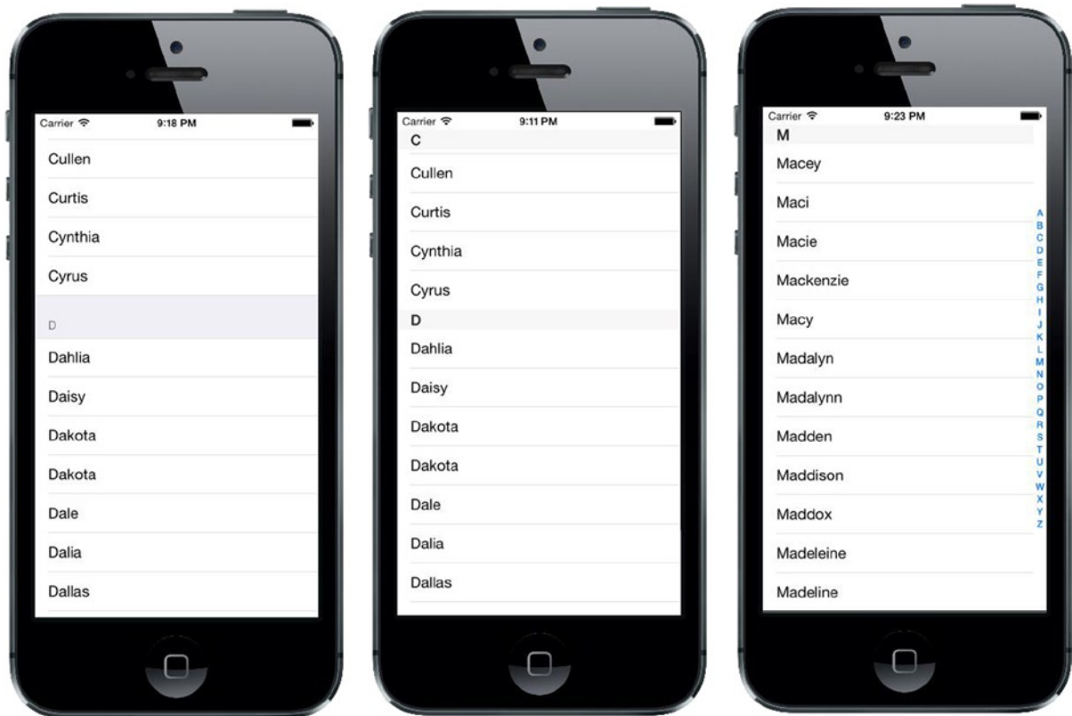
Figure 8-3. The same table view displayed as a grouped table (left); a plain table without an index (middle); and a plain table with an index, which is also called an indexed table (right)
