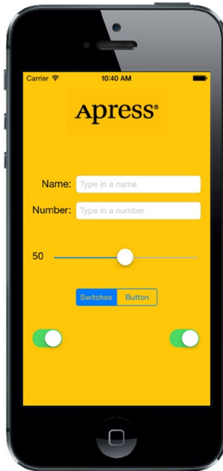
Figure 4-1. The Control Fun application features text fields, labels, a slider, and several other stock iPhone controls
