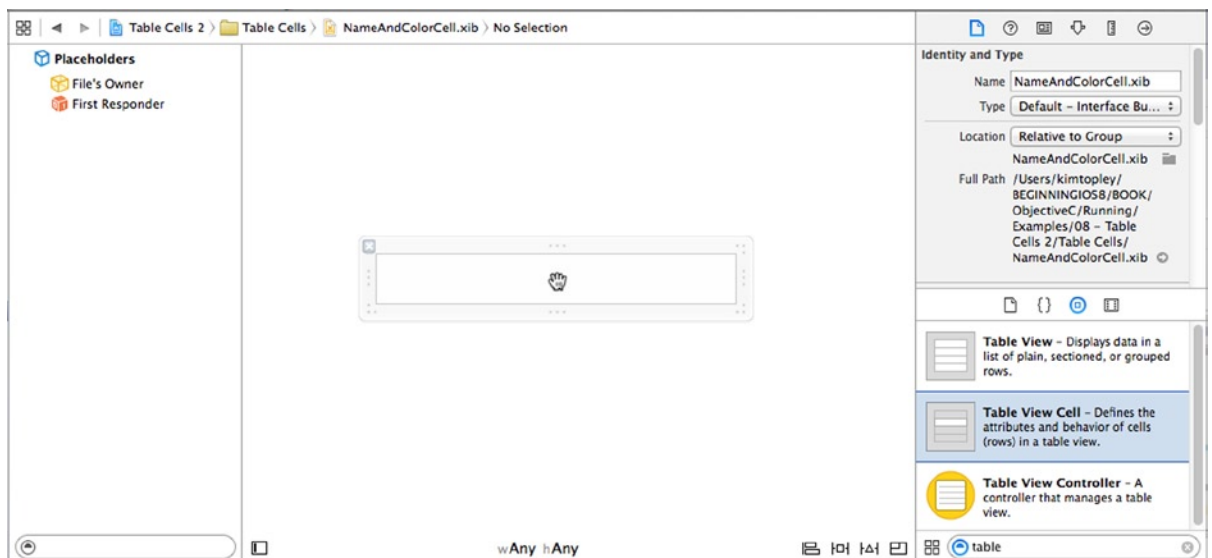
Figure 8-18. We dragged a table view cell from the library into the nib editor
