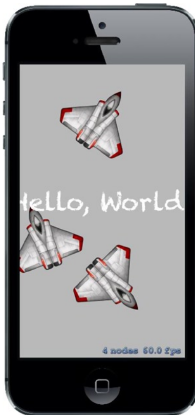
Figure 17-1. The default Sprite Kit app in action. Some text is displayed in the center of the screen, and each tap on the screen puts a rotating graphic of a fighter jet at that location
