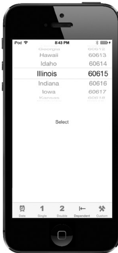
Figure 7-5. In this picker, one component is dependent on the other. As you select a state in the left component, the right component changes to a list of ZIP codes in that state
