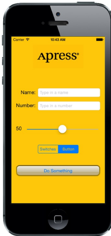
Figure 4-2. Tapping the segmented controller on the left side causes a pair of switches to be displayed. Tapping the right side causes a button to be displayed
