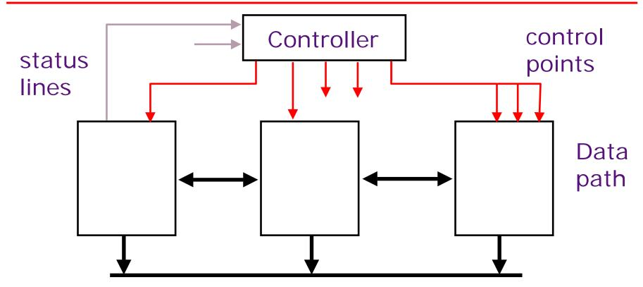
*Structure:* How components are connected. *Static Behavior:* How data moves between components *Dynamic*
