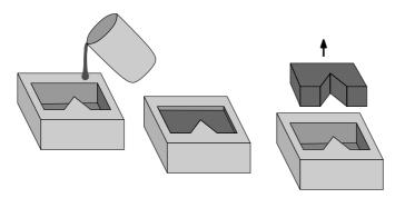
Figure 4.1 The casting process
