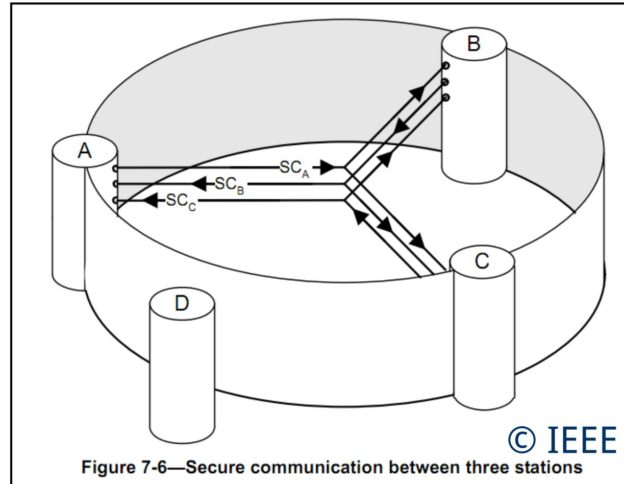
Figure 7-6—Secure communication between three stations
