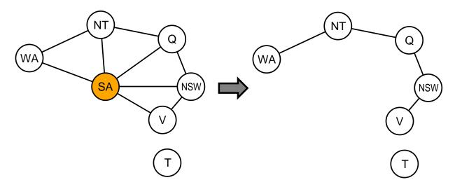
Cutset conditioning: instantiate (in all ways) a set of variables such that the remaining constraint graph is a tree
