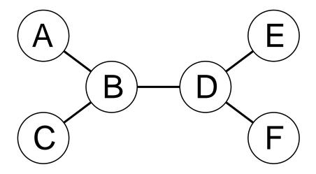
Theorem: if the constraint graph has no loops, the CSP can be solved in  $O(n\,d^2)$  time
