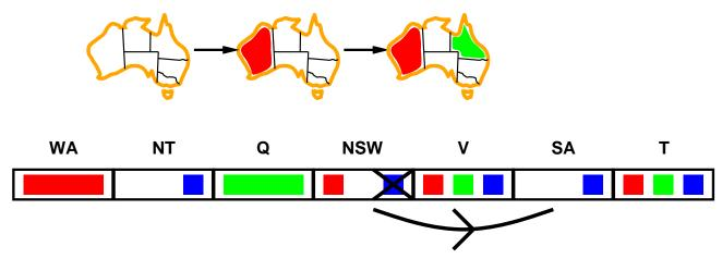
Simplest form of propagation makes each arc consistent
