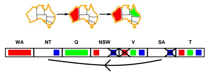
If X loses a value, neighbors of X need to be rechecked Arc consistency detects failure earlier than forward checking Can be run as a preprocessor or after each assignment
